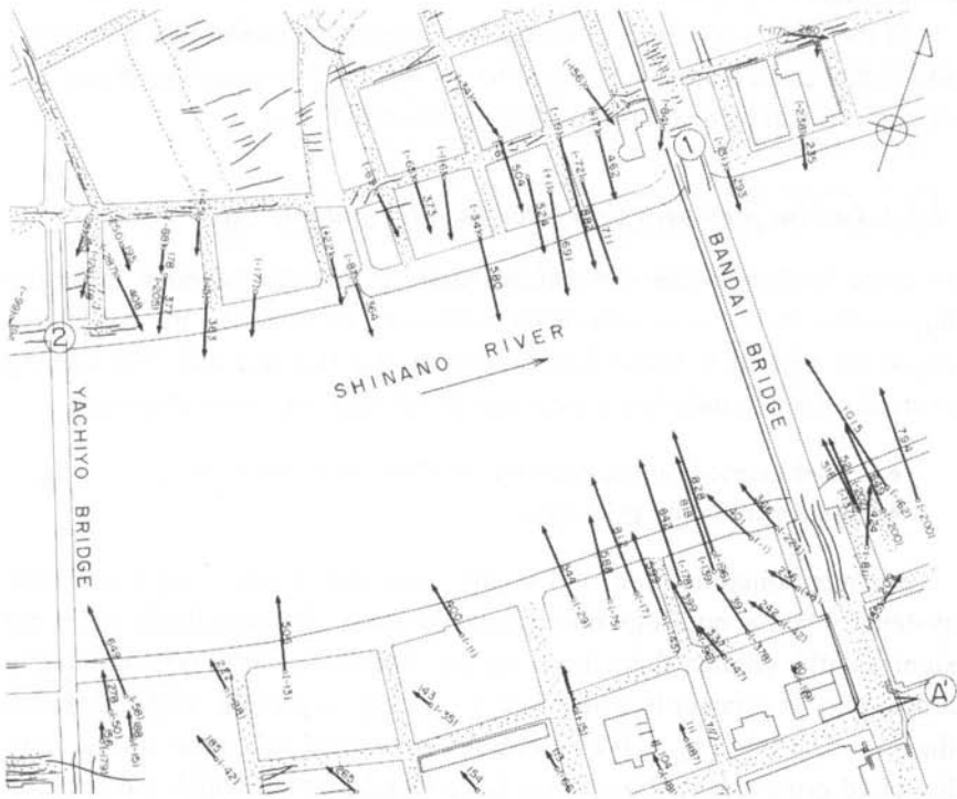
Fig. 4.7 Ground movements in cm in Niigata during the 1964 Earthquake. (Hamada, 1992).
