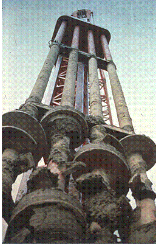
Figure 142. Photo. Typical auger-based tools for WRS methods.
