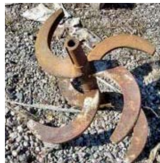
Figure 152. Photo. Typical mixing tool for DRE methods for peat mixing. (118)
