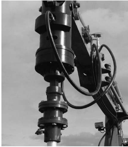
Figure 2.17 TorqueMaster device (Courtesy of Magnum Piering, Inc.)
