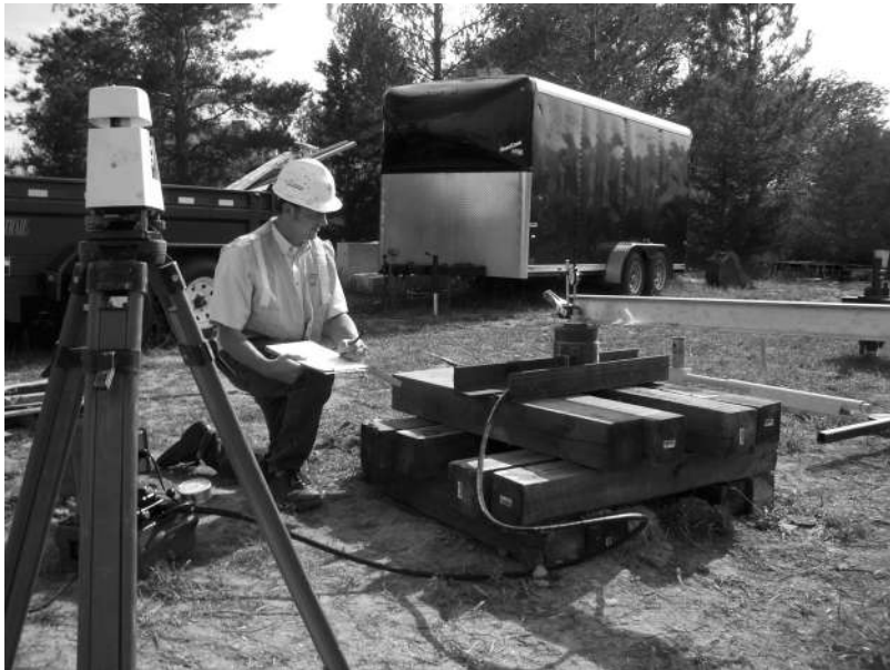
Figure 7.6 Helical pile tension test
