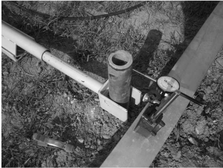
Figure 10.11 Dial gage used to measure lateral displacements
