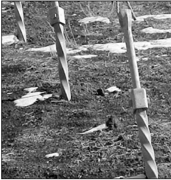
Figure 2.23 Twisted helical anchor shafts (Downey, 2008)
