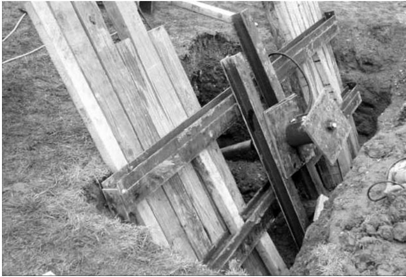
Figure 7.5 Performance test on a helical anchor (Courtesy of Magnum Piering, Inc.)
