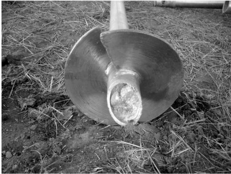
Figure 4.12 Plugged end of a typical helical pile
